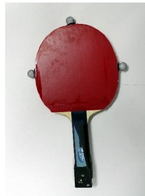
Figure 1. Racket and an attached inertial sensor
