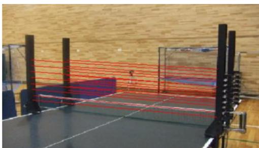
**Fig.1** The system of the two infrared sensors was fixed 0.3 m from the net respectively.
