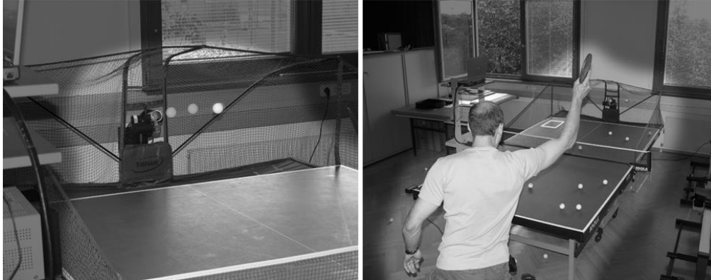
Figure 5 Feedback training using impact position detecting system
